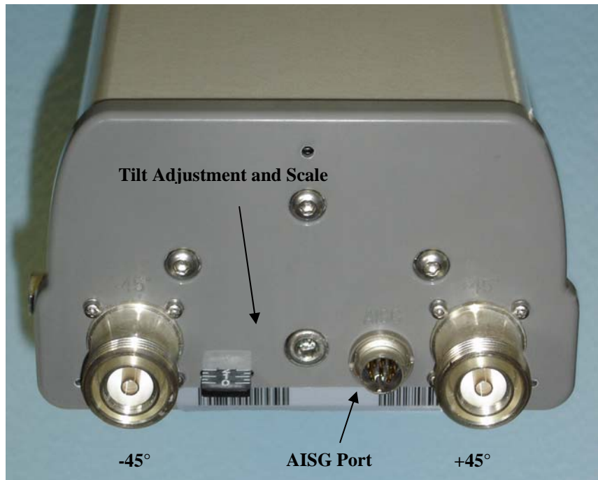
Figure 9. AISG Compliant Adjustable Downtilt Antenna showing Hex Socket for Manual Adjustment and Horizontal Angle Indicator Scale protruding past face of base.
