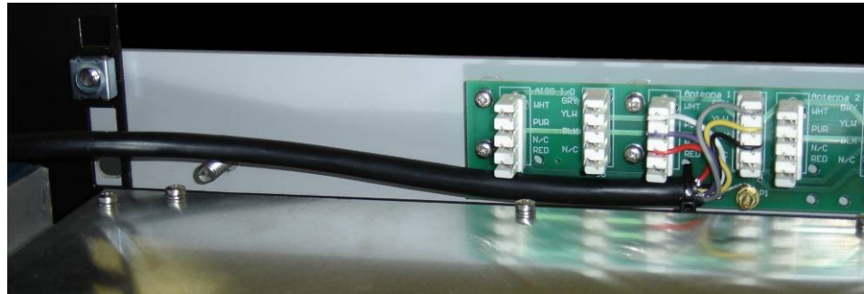
Figure 3. Properly Run Cable for Rack Mounting.
